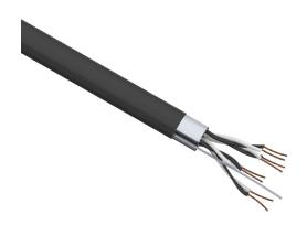
Quabbin instrumentation cable, overall shielded, PLTC and ITC, 300V, 4 twisted pairs, 18 AWG, PVC conductor insulation material, black and white numbered pairs, PVC jacket, black, cut to length.
