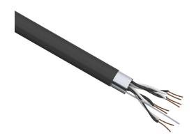
Quabbin instrumentation cable, overall shielded, PLTC and ITC, 300V, 4 twisted pairs, 18 AWG, PVC conductor insulation material, black and white numbered pairs, PVC jacket, black, cut to length.
