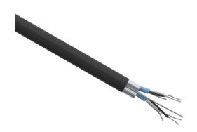
Quabbin instrumentation cable, individual and overall shielded, PLTC and ITC, 300V, 2 twisted pairs, 18 AWG, PVC conductor insulation material, black and white numbered pairs, PVC jacket, black, cut to length.
