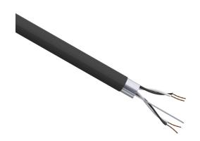
Quabbin instrumentation cable, overall shielded, PLTC and ITC, 300V, 2 twisted pairs, 18 AWG, PVC conductor insulation material, black and white numbered pairs, PVC jacket, black, cut to length.
