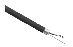
Quabbin instrumentation cable, overall shielded, PLTC and ITC, 300V, 1 twisted pair, 18 AWG, PVC conductor insulation material, black and white numbered pairs, PVC jacket, black, cut to length.
