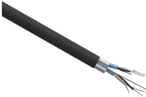
Quabbin instrumentation cable, individual and overall shielded, PLTC and ITC, 300V, 2 twisted pairs, 16 AWG, PVC conductor insulation material, black and white numbered pairs, PVC jacket, black, cut to length.
