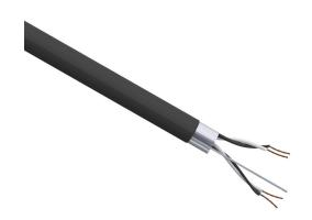
Quabbin instrumentation cable, overall shielded, PLTC and ITC, 300V, 2 twisted pairs, 16 AWG, PVC conductor insulation material, black and white numbered pairs, PVC jacket, black, cut to length.
