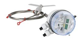
ProSense rotating paddle bulk solids level switch, 2000mm rope insertion length, 1-1/4in male NPT process connection, (1) SPDT relay, 20-28 VDC operating voltage. Hinged paddle included.
