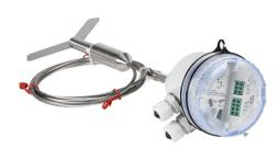
ProSense rotating paddle bulk solids level switch, 2000mm rope insertion length, 1-1/4in male NPT process connection, (1) SPDT relay, 230 VAC operating voltage. Hinged paddle included. Hazardous location rated.
