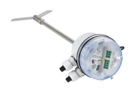
ProSense rotating paddle bulk solids level switch, 300mm insertion length, 1-1/4in male NPT process connection, (1) SPDT relay, 20-28 VDC operating voltage. Hinged paddle included.
