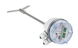
ProSense rotating paddle bulk solids level switch, 300mm insertion length, 1-1/4in male NPT process connection, (1) SPDT relay, 20-28 VDC operating voltage. Hinged paddle included. Hazardous location rated.
