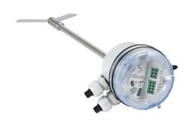
ProSense rotating paddle bulk solids level switch, 300mm insertion length, 1-1/4in male NPT process connection, (1) SPDT relay, 230 VAC operating voltage. Hinged paddle included.
