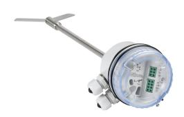
ProSense rotating paddle bulk solids level switch, 300mm insertion length, 1-1/4in male NPT process connection, (1) SPDT relay, 230 VAC operating voltage. Hinged paddle included. Hazardous location rated.
