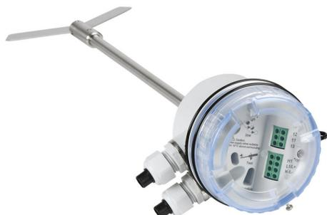
ProSense rotating paddle bulk solids level switch, 300mm insertion length, 1-1/4in male NPT process connection, (1) SPDT relay, 115 VAC operating voltage. Hinged paddle included.
