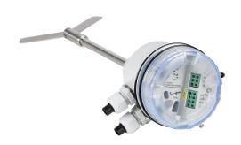
ProSense rotating paddle bulk solids level switch, 200mm insertion length, 1-1/4in male NPT process connection, (1) SPDT relay, 20-28 VDC operating voltage. Hinged paddle included.
