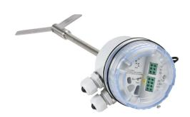
ProSense rotating paddle bulk solids level switch, 200mm insertion length, 1-1/4in male NPT process connection, (1) SPDT relay, 20 to 28 VDC operating voltage. Hinged paddle included. Hazardous location rated.
