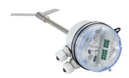
ProSense rotating paddle bulk solids level switch, 200mm insertion length, 1-1/4in male NPT process connection, (1) SPDT relay, 230 VAC operating voltage. Hinged paddle included. Hazardous location rated.
