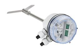
ProSense rotating paddle bulk solids level switch, 200mm insertion length, 1-1/4in male NPT process connection, (1) SPDT relay, 115 VAC operating voltage. Hinged paddle included.
