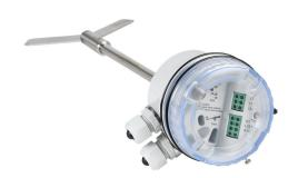
ProSense rotating paddle bulk solids level switch, 200mm insertion length, 1-1/4in male NPT process connection, (1) SPDT relay, 115 VAC operating voltage. Hinged paddle included. Hazardous location rated.
