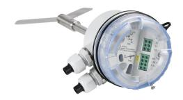
ProSense rotating paddle bulk solids level switch, 100mm insertion length, 1-1/4in male NPT process connection, (1) SPDT relay, 20 to 28 VDC operating voltage. Hinged paddle included.
