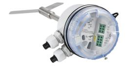
ProSense rotating paddle bulk solids level switch, 100mm insertion length, 1-1/4in male NPT process connection, (1) SPDT relay, 20-28 VDC operating voltage. Hinged paddle included.
