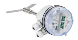
ProSense rotating paddle bulk solids level switch, 100mm insertion length, 1-1/4in male NPT process connection, (1) SPDT relay, 230 VAC operating voltage. Hinged paddle included. Hazardous location rated.
