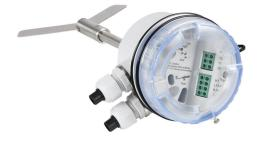
ProSense rotating paddle bulk solids level switch, 100mm insertion length, 1-1/4in male NPT process connection, (1) SPDT relay, 115 VAC operating voltage. Hinged paddle included.
