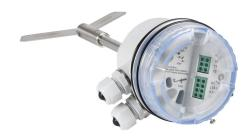
ProSense rotating paddle bulk solids level switch, 100mm insertion length, 1-1/4in male NPT process connection, (1) SPDT relay, 115 VAC operating voltage. Hinged paddle included. Hazardous location rated.
