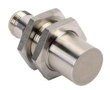
ProSense inductive proximity sensor, tubular, 18mm diameter x 45mm body, stainless steel housing, PNP, N.O. output, 12mm sensing distance, non-flush, 250 Hz switching frequency, IP65 IP66 IP67 IP68 IP69K, 4-pin M12 quick-disconnect.
