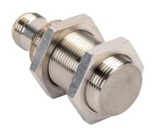
ProSense inductive proximity sensor, tubular, 18mm diameter x 45mm body, stainless steel housing, PNP, N.O. output, 8mm sensing distance, flush, 100 Hz switching frequency, IP65 IP66 IP67 IP68 IP69K, 4-pin M12 quick-disconnect.
