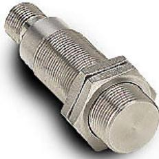
AutomationDirect inductive proximity sensor, tubular, 18mm diameter x 63.5mm body, stainless steel housing, PNP, N.O. output, 10mm sensing distance, flush, 200 Hz switching frequency, IP67, 4-pin M12 quick-disconnect.
