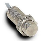
AutomationDirect inductive proximity sensor, tubular, 18mm diameter x 63.5mm body, stainless steel housing, PNP, N.O. output, 10mm sensing distance, flush, 200 Hz switching frequency, IP68, pigtail.
