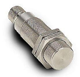
AutomationDirect inductive proximity sensor, tubular, 18mm diameter x 63.5mm body, stainless steel housing, NPN, N.O. output, 10mm sensing distance, flush, 200 Hz switching frequency, IP67, 4-pin M12 quick-disconnect.
