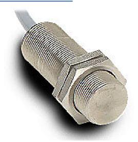
AutomationDirect inductive proximity sensor, tubular, 18mm diameter x 63.5mm body, stainless steel housing, NPN, N.O. output, 10mm sensing distance, flush, 200 Hz switching frequency, IP68, pigtail.
