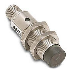
Micro Detectors inductive proximity sensor, tubular, 18mm diameter x 63.5mm body, stainless steel housing, PNP, N.O./N.C. complementary outputs, 8mm sensing distance, non-flush, 1 kHz switching frequency, IP67 IP68, 4-pin M12 quick-disconnect.
