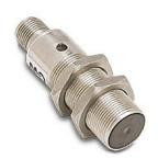
Micro Detectors inductive proximity sensor, tubular, 18mm diameter x 63.5mm body, stainless steel housing, PNP, N.O./N.C. complementary outputs, 5mm sensing distance, flush, 1 kHz switching frequency, IP67 IP68, 4-pin M12 quick-disconnect.
