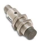
Micro Detectors inductive proximity sensor, tubular, 18mm diameter x 63.5mm body, stainless steel housing, NPN, N.O./N.C. complementary outputs, 8mm sensing distance, non-flush, 1 kHz switching frequency, IP67 IP68, 4-pin M12 quick-disconnect.
