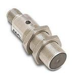
Micro Detectors inductive proximity sensor, tubular, 18mm diameter x 63.5mm body, stainless steel housing, NPN, N.O./N.C. complementary outputs, 5mm sensing distance, flush, 1 kHz switching frequency, IP67 IP68, 4-pin M12 quick-disconnect.
