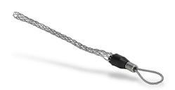
Bryant junior pulling grip, low tension, accepts cable diameter size 1 to 1.24in, closed single weave, galvanized steel mesh, 11.5in length, flexible, eye length 6-1/2in.
