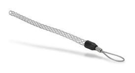
Bryant junior pulling grip, low tension, accepts cable diameter size 0.5 to 0.61in, closed single weave, galvanized steel mesh, 8.5in length, flexible, eye length 4-1/4in.
