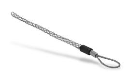
Bryant junior pulling grip, low tension, accepts cable diameter size 0.37 to 0.49in, closed single weave, galvanized steel mesh, 7in length, flexible, eye length 3-3/4in.
