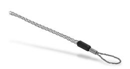
Bryant junior pulling grip, low tension, accepts cable diameter size 0.25 to 0.36in, closed single weave, galvanized steel mesh, 4.25in length, flexible, eye length 3-1/4in.
