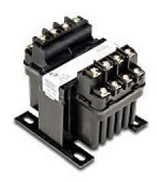
Hammond control transformer, encapsulated core, 75 VA, 1-phase, 120/240 VAC primary, 12/24 VAC secondary, 50/60 Hz, panel mount.
