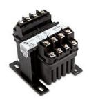
Hammond control transformer, encapsulated core, 75 VA, 1-phase, 240/480 VAC primary, 120/240 VAC secondary, 50/60 Hz, panel mount.
