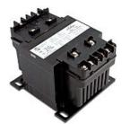
Hammond control transformer, encapsulated core, 750 VA, 1-phase, 240/480 VAC primary, 120/240 VAC secondary, 50/60 Hz, panel mount.
