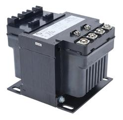
Hammond control transformer, encapsulated core, 750 VA, 1-phase, 240/480 VAC primary, 25/120 VAC secondary, 50/60 Hz, panel mount.
