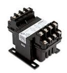
Hammond control transformer, encapsulated core, 50 VA, 1-phase, 240/480 VAC primary, 120/240 VAC secondary, 50/60 Hz, panel mount.
