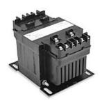
Hammond control transformer, encapsulated core, 500 VA, 1-phase, 240/480 VAC primary, 25/120 VAC secondary, 50/60 Hz, panel mount.
