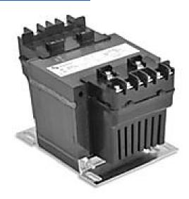
Hammond control transformer, encapsulated core, 500 VA, 1-phase, 208/277/380 VAC primary, 120/240 VAC secondary, 50/60 Hz, panel mount.
