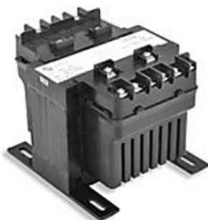
Hammond control transformer, encapsulated core, 350 VA, 1-phase, 240/480 VAC primary, 25/120 VAC secondary, 50/60 Hz, panel mount.
