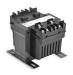
Hammond control transformer, encapsulated core, 350 VA, 1-phase, 208/277/380 VAC primary, 120/240 VAC secondary, 50/60 Hz, panel mount.
