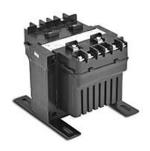
Hammond control transformer, encapsulated core, 250 VA, 1-phase, 240/480 VAC primary, 25/120 VAC secondary, 50/60 Hz, panel mount.
