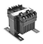
Hammond control transformer, encapsulated core, 250 VA, 1-phase, 208/277/380 VAC primary, 120/240 VAC secondary, 50/60 Hz, panel mount.
