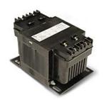
Hammond control transformer, encapsulated core, 1.5 kVA, 1-phase, 240/480 VAC primary, 120/240 VAC secondary, 50/60 Hz, panel mount.
