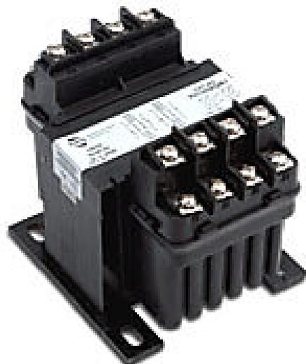
Hammond control transformer, encapsulated core, 100 VA, 1-phase, 240/480 VAC primary, 120/240 VAC secondary, 50/60 Hz, panel mount.
