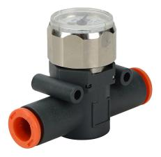
NITRA pneumatic push-to-connect fitting, inline pressure gauge, technopolymer body, (1) 5/16in (8mm) push-to-connect inlet(s), (1) 5/16in (8mm) push-to-connect outlet(s), 0-170 psi range.
